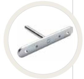
**SHELF SUPPORT (Heavy Duty 16mm rebar)** Made from 16mm solid steel bar. Suitable for shelf depths of 145–500mm. Each support will hold up to 25kg at 150mm shelf depth. Supplied with resin. Permanent bond.
