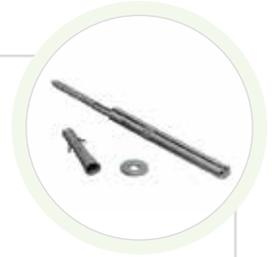
**SHELF SUPPORT (Adjustable 14mm Triade)** Made from steel & alloy and fully adjustable in all directions. Fix directly to the wall or use with the optional shelf support bracket. Suitable for shelf depths of 185–300mm. Each support will hold up to 15kg at 185mm shelf depth.
