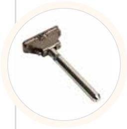
**SHELF SUPPORT BRACKET (for use with 14mm Triade)** Provides extra strength for the triade shelf support if required. Made from steel and locates into the wall with a steel pin via a drilled hole and fixes with wall screws, triade shelf support can then be fixed to the wall bracket to give optimum support and also prevent tipping.
